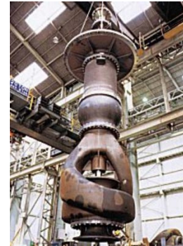
One of the 20 vertical mixed-flow brine re-circulation pumps. In all, over 100 pumps of varying designs and sizes were used in the plant (© Copyright 2009 SPG Media Limited)
