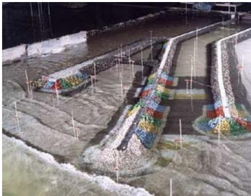
Model test of marine outfall structures (COWI Marine and coastal engineering)
