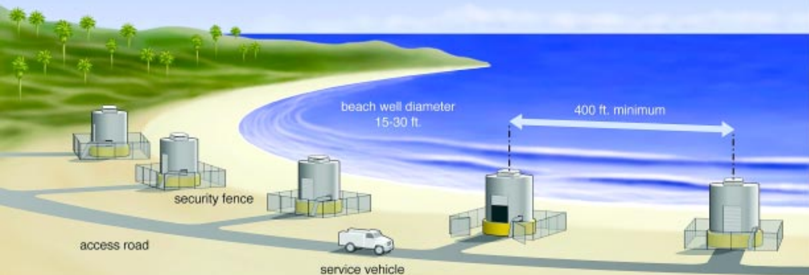
Figure 1 - Beach Well Intake System – Impact on the Seashore
