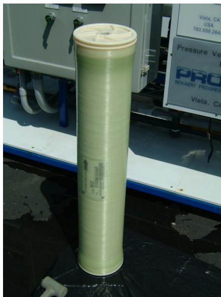
Figure 19 – Typical 8-inch Membrane Element
