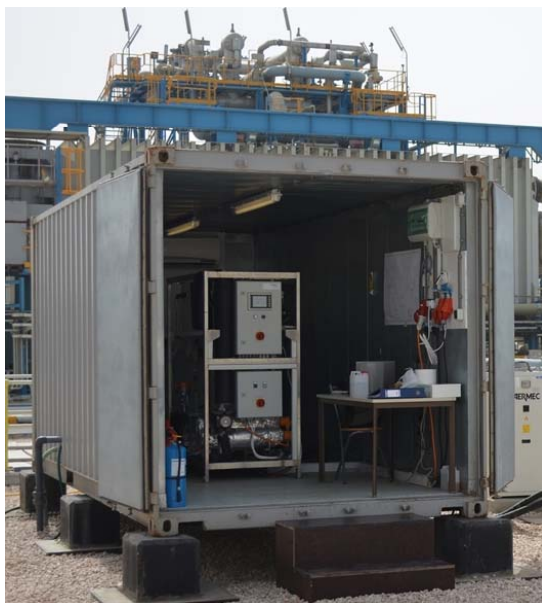
Project will use a Vacuum-MD pilot unit for the testing.
