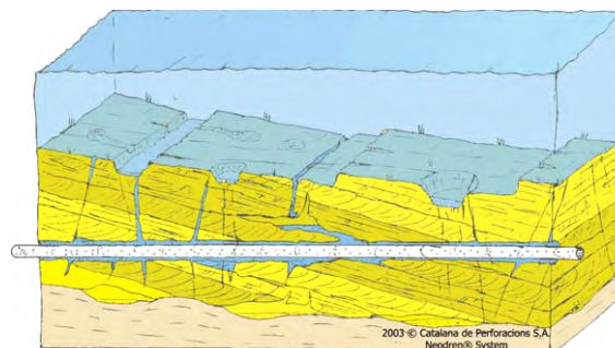
Fig. 1. Horizontal drain in the sea bed.
