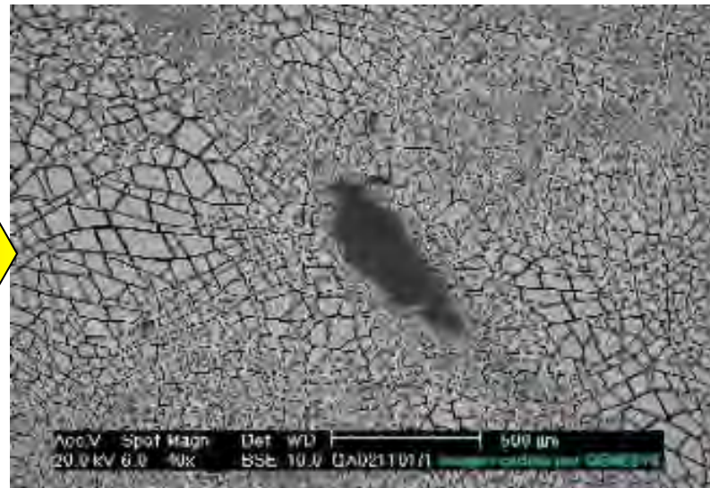
SEM-EDAX micrograph of calcium phosphate deposit
