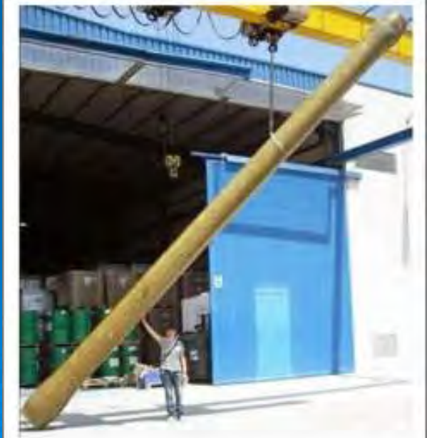
BEL's 16-inch diameter, 8-element Pressure Vessel
