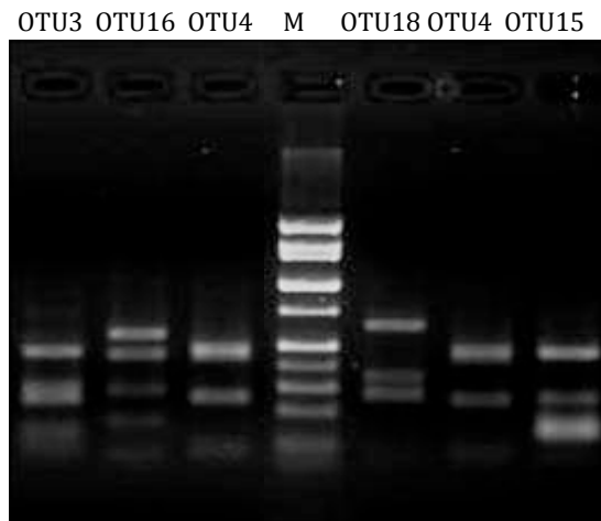
Figure 4-1. Restriction fragment length polymorphism analysis of 16S rRNA gene clone library of RO membrane biofilm revealing different patterns among clones. Five operational taxonomic units (OTUs) are presented in the picture.
