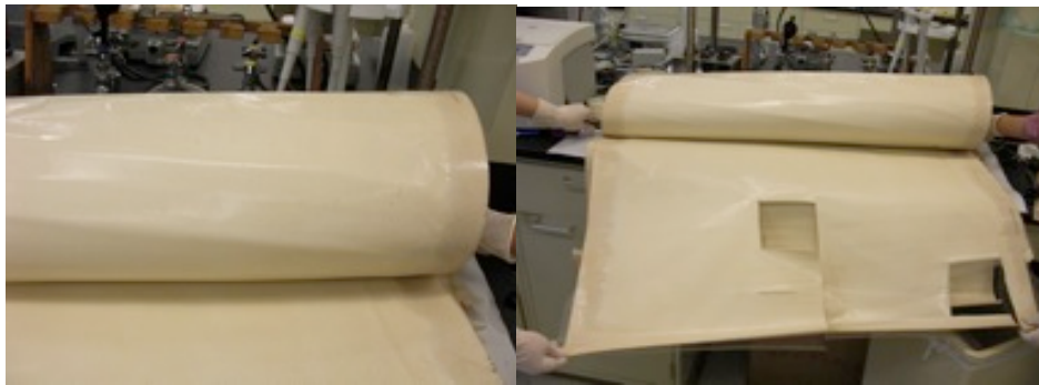
Figure 9-1. The RO membrane from West Basin plant chloramines study. The feed end of the RO membrane is shown on the left with sparse brown particulates. The same membrane element after excision is shown on the right.
