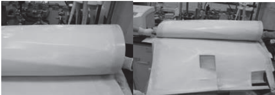
Figure 9.1. RO membrane from West Basin plant chloramines study.
