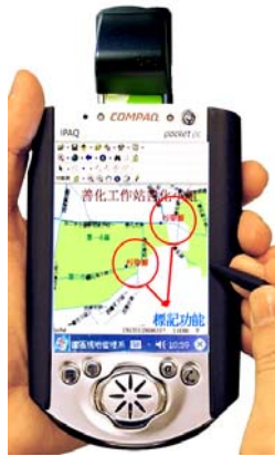
Fig. 7 Mobil GIS integrating PDA, GIS and GPS
