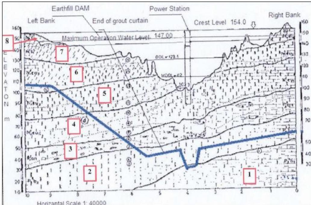
Figure 9: Geological cross section under Haditha Dam, showing the lower limits of the grout curtain. Note that the karstification is developed in the Lower Member of the Euphrates Formation (Units 3, 4 and 5), underlain by the cavernous Anah Formation (Unit 2).
