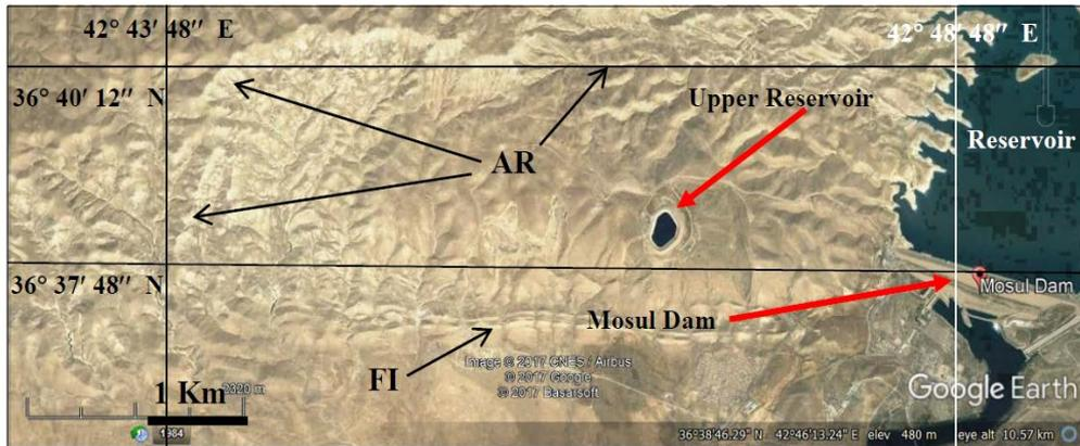
Figure 2: Google Earth image of Mosul Dam site. Note the anticlinal ridges (AR) and the Flat irons (FI)
