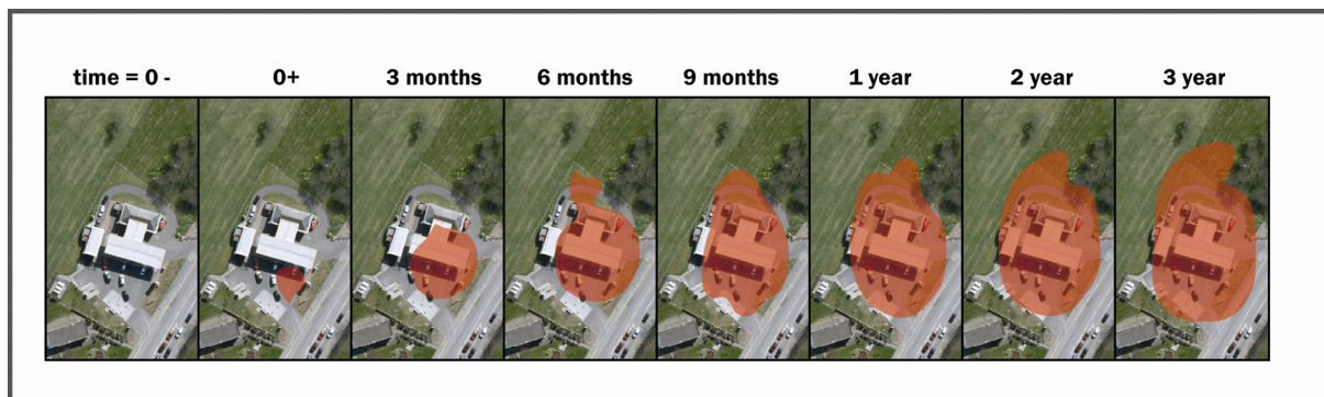
Figure 6.2. LNAPL release of fuel oil observed in monitoring wells showing that lateral stability was largely achieved within the first year of the release with reduced lateral expansion in years two and three. Lighter LNAPLs tend to reach lateral stability quicker (months), whereas heavier more viscous LNAPLs (such as Fuel Oil No.6) may require several years to attain stability (API, 2004). Decreasing saturation, LNAPL gradients and entry pressures retard the growth of the LNAPL source area resulting in its ultimate stabilisation.
