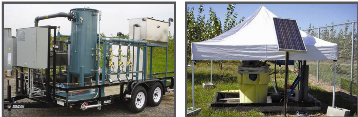
Figure 7.6. Examples of site remediation systems showing a multi-phase extraction unit (left) and a solar-powered belt skimmer at a Superfund site in the eastern USA (Photographs courtesy of B. Butler, ERM).
