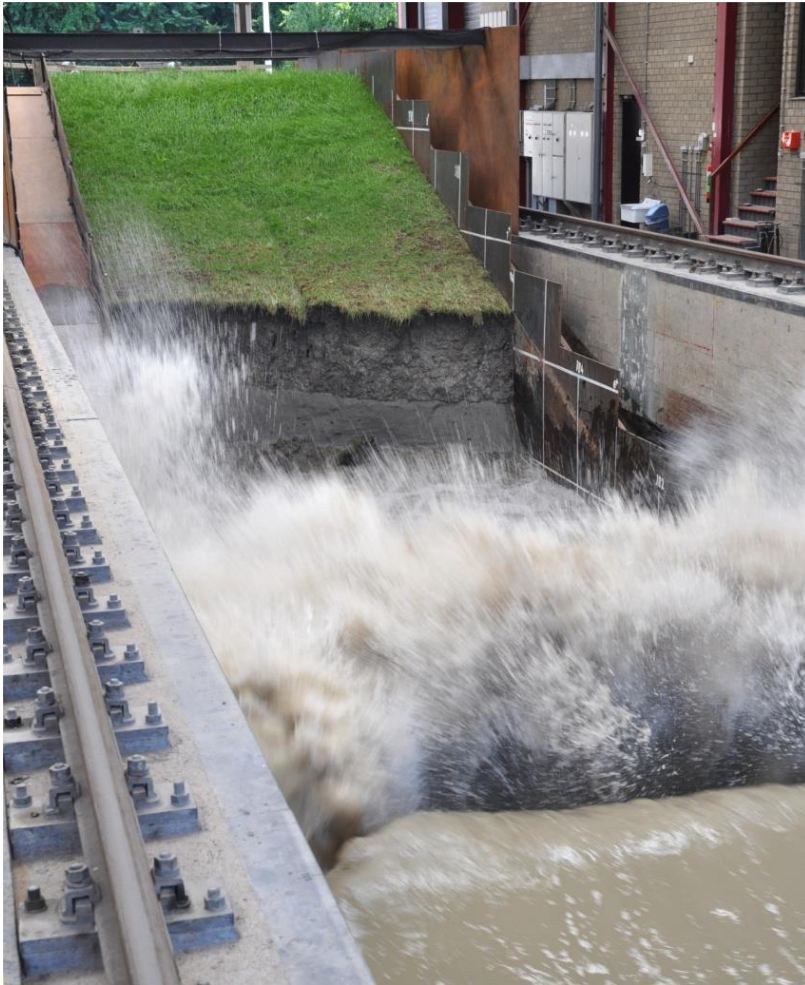
Erosion of the clay layer and the sand core by waves
