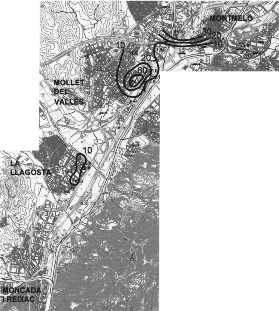
Fig. 6. Iso PCE+TCE concentration map of the La Llagosta alluvial aquifer unit (values in ppb) and location of sampling points with high amounts of dense chlorinated solvents.
