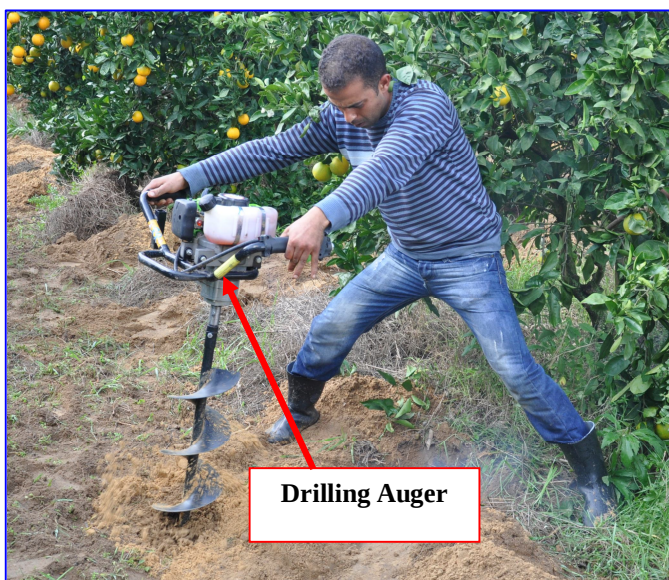
Use of drilling auger to prepare the pits (holes) for the installation of the buried diffusers for orange trees in Beni Khalled , Cap Bon North of Tunisia
