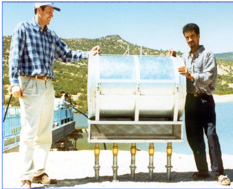
Big sized draining floater for big dams and rivers
