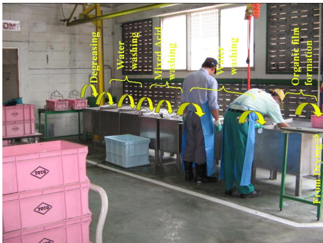
Fig.2 Our surface treatment process in Thailand
