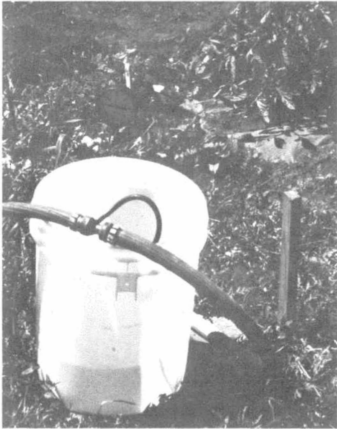
14 Figure 13. Inexpensive "hoze-on" proportioner roughly 1 to 20 dilution, varying with pressure and flow.
