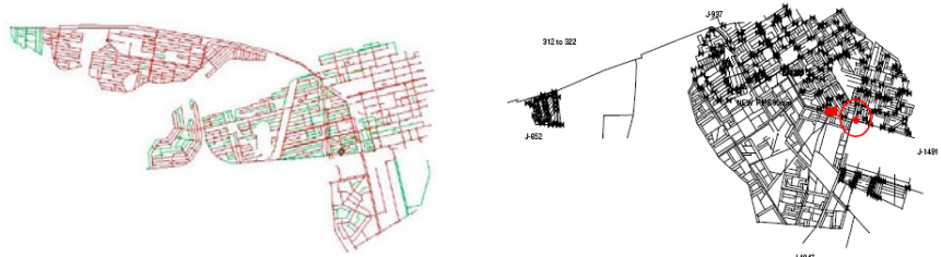
GIS representation of supply area R7 (left) and EPANET critical point identification in supply area RE (right)
