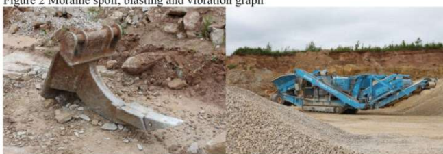
Figure 3 Ripper and crusher
