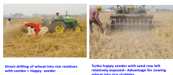
Fig 4 Happy Seeder for Zero Tilled wheat to improve water productivity
