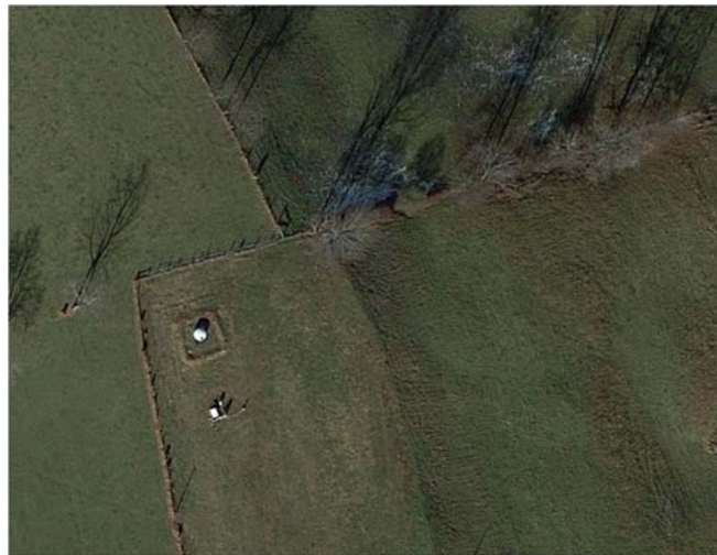
Figure 2.4 Potential source of contamination: oil or gas well. (Note the nearby above ground storage tank with earthen berm for secondary containment).
