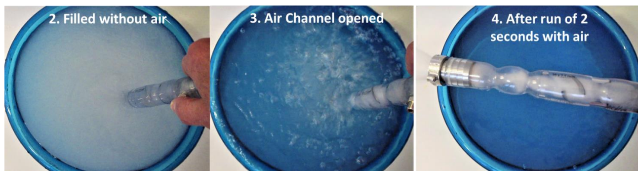
Fig. 5 Separated and activated tap water left, two second post-clarification of the activated tap water with OxTube and air suction middle, Clarification and Dissolving of two seconds with OxTube Integrated Clarification and air right.
