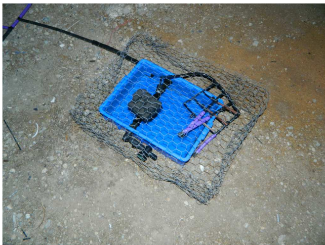
A chicken wire cage protected the evaporator from birds and other animals
