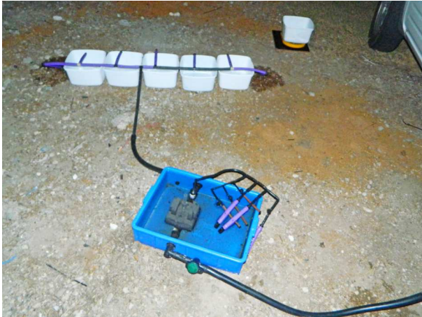
Research trials at Adelaide Airport using the Unpowered Measured Irrigation Controller
