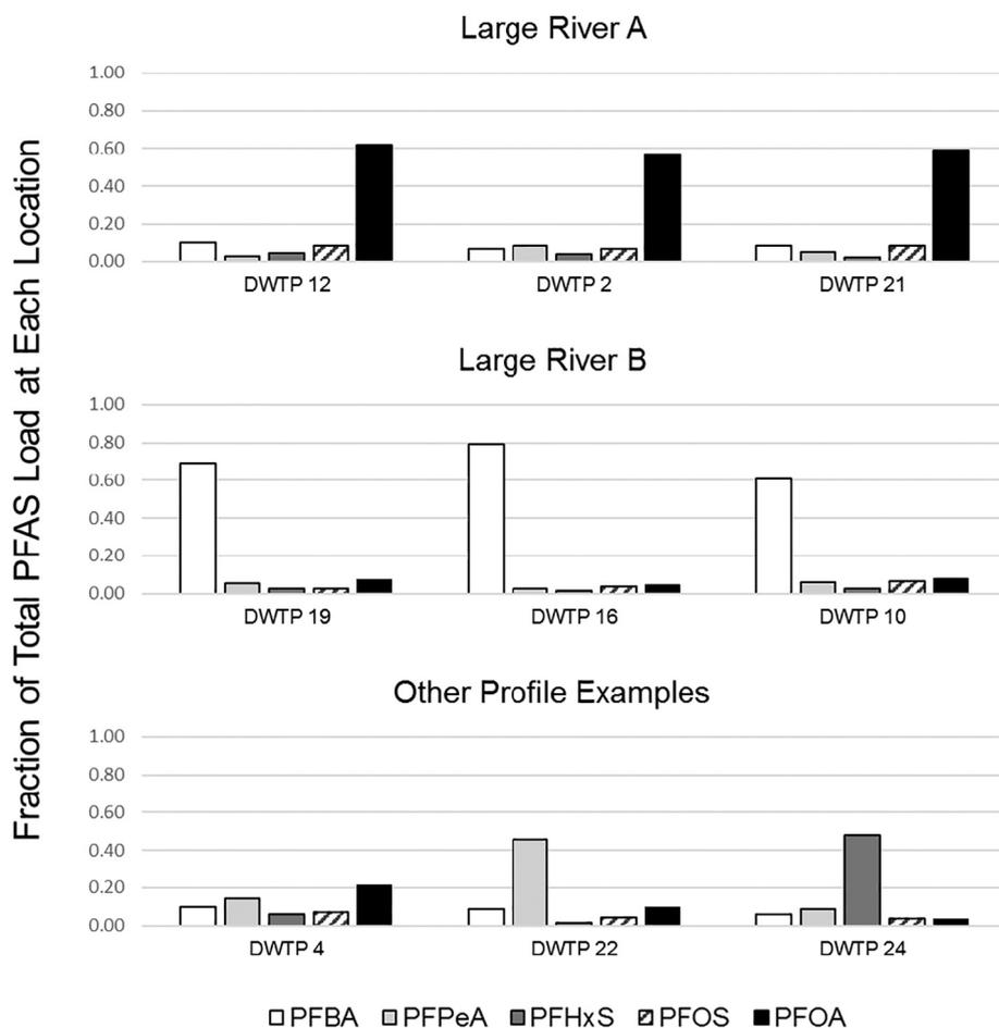
Fig. 2. PFAS analyte patterns along two rivers. Locations for Large Rivers A and B are ordered by river flow progressing left to right. Other Profile Examples are not related to each other.
