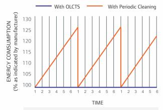
The area bounded by the orange line represents the potential power conservation (up to 30%). This is a significant saving considering that HVAC accounts for approximately 60% of the total electrical consumption of a large building.
