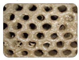
"Fouling" is an undesirable pile deposit formed inside condenser tubes, sometimes described as thermal resistant on the heat path in the condenser.
