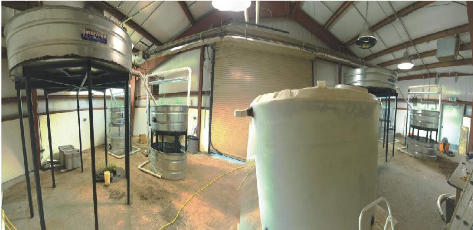
Figure 3.1: Detailed image of 1500 gallon water storage tank, sedimentation tanks, recycled vertical flow constructed wetland (RVFCW) units, RVFCW reservoirs, RVFCW grow lights, and effluent distribution pipes.
