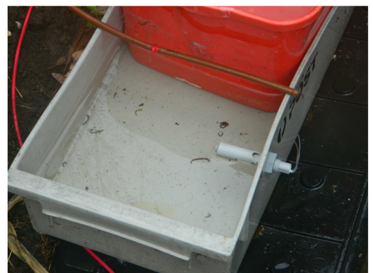
Evaporator for Garden Bed 2 showing the control dripper and a surface area of evaporation of 0.52 \text{ m}^2 .
