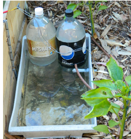
The surface area of evaporation may be reduced by placing full bottles of water in the evaporator.
