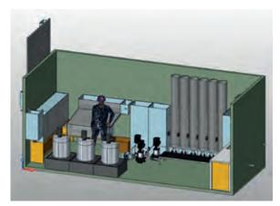
3D model of a water characterisation unit designed by OiEau @OiEau
