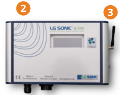
Control box to select treatment program
