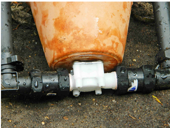
Unpowered Terracotta Irrigation Controller showing the valve and the 15mm inlet and outlet
