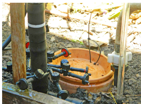
Fraction 1/4 for online dripper (4 closed lower drippers, 4 open lower drippers and one open lower dripper as control dripper) water supply pressure 100 kPa
