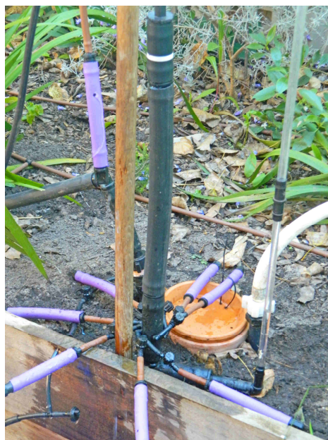
Fraction 1/2 for 13mm dripline (4 closed lower drippers, 4 open lower drippers and 2 open lower drippers as control dripper) water supply pressure 100 kPa
