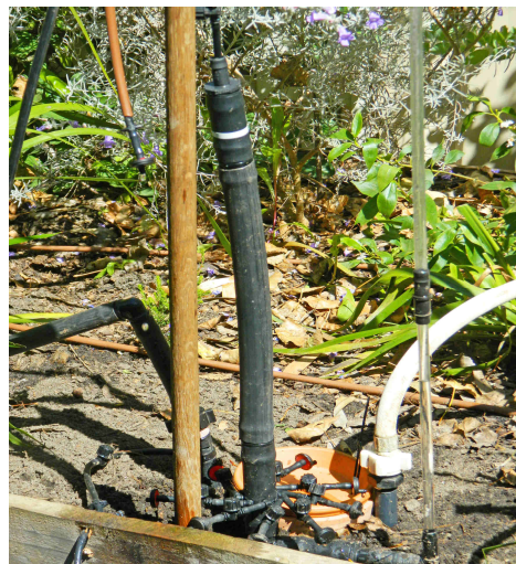
Fraction 1/8 for online dripper, water supply pressure 100 kPa. The extension tube is used so that the water level showing in the clear tube is below the white line.
