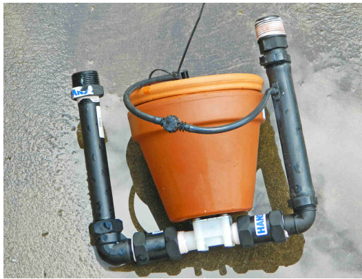
Step 1. Adjust the inlet and outlet pipes so that they are vertical.
