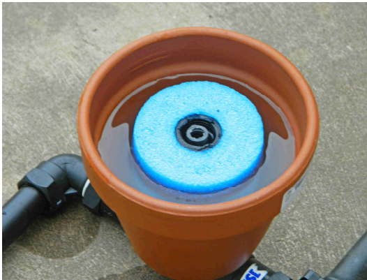
Unpowered Terracotta Irrigation Controller showing the float and the water level
