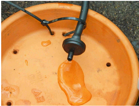
The adjustable control dripper has been replaced by an on-line irrigation dripper.
