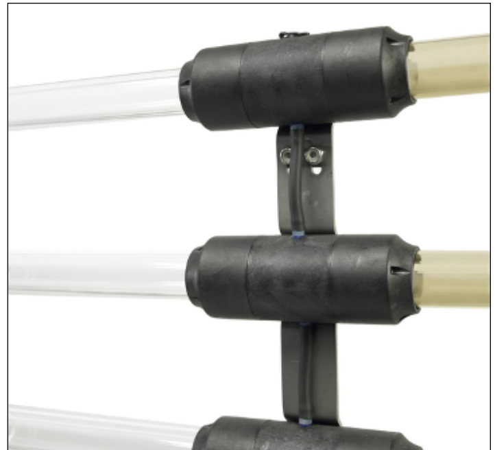
UV lamps in TrojanUV systems are enclosed in a quartz sleeve to insulate them from the water. ActiClean™ is our patented dual-action sleeve cleaning system that uses mechanical wiping in conjunction with ActiClean Gel contained within wiper canisters surrounding the quartz sleeves.
