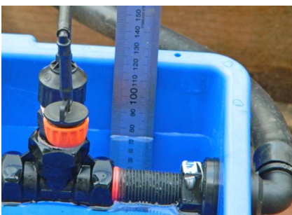
Measure the depth of water in the evaporator at the low level
