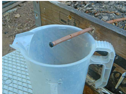
Remove water from the evaporator until the irrigation starts
