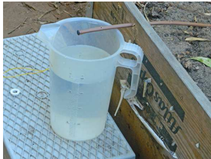
Dripper control volume in the measuring container
