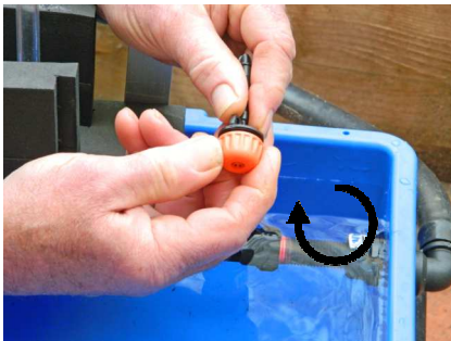
If volume in the measuring container is less than the dripper control volume, turn the control dripper clockwise to reduce the flow rate of the control dripper.
