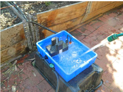
Fill the evaporator with water until the water level reaches the high level
