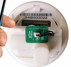
LPWAN telemetry equipped water meter
