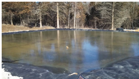
Figure 10. Buick Mine 10 gpm SRB pilot test, 2011. Note rock sitting on 2-inch ice layer. SRB biocell was producing 3 mg/L residual sulfide at water temperature of 4° C and removing Zn to <100 µg/L.
