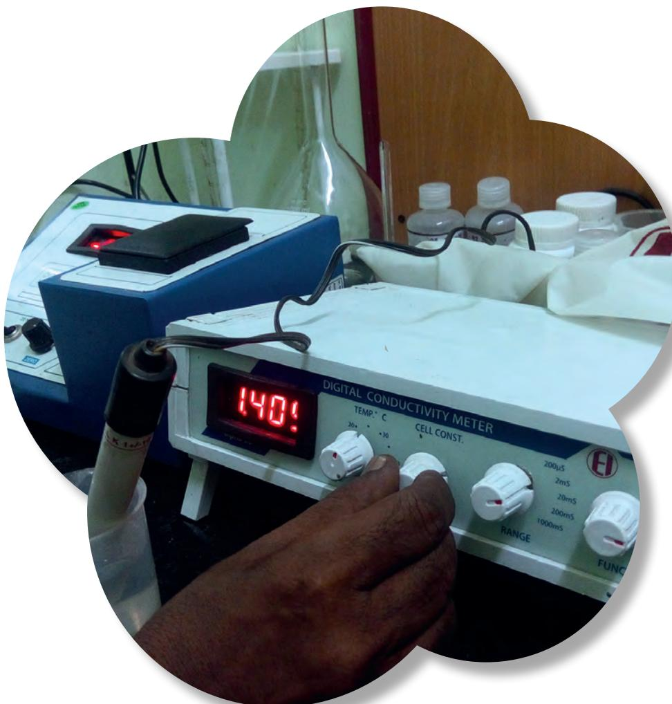
Apparatus for conductivity test
