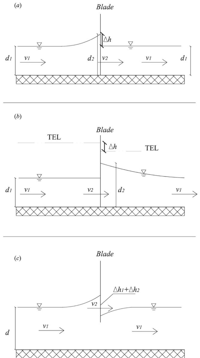
**Fig. 5.** Hydraulic behavior of stream wheels and theoretical energy transfer between the water flow and the blades of the wheel. (a) Stream water wheel in subcritical shallow water (b) stream water wheel in supercritical shallow water, (c) stream water wheel in deep (subcritical) water.  $v_1$  is the undisturbed flow velocity, while  $v_2$  is the blade velocity
