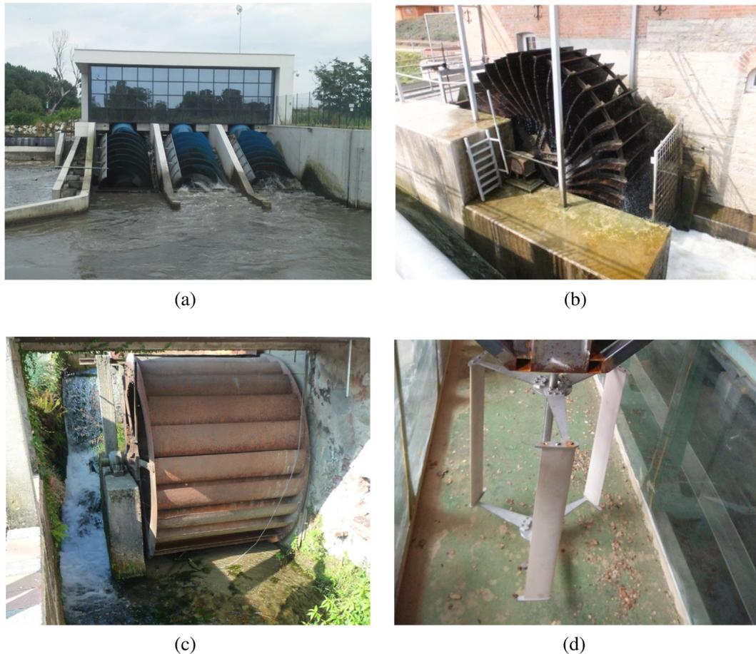
**Fig. 1.** (a) Three Archimedes screw in parallel (Enerca power plant, Crescenzago, Italy, photo of Emanuele Quaranta), (b) undershot water wheel (Germany, photo of Gerald Müller), (c) overshot water wheel, research project ORME (Ciconio, Italy) (Quaranta, 2017) and (d) Darrieus hydrokinetic turbine (installed in the Hydraulic laboratory of Politecnico di Torino).
