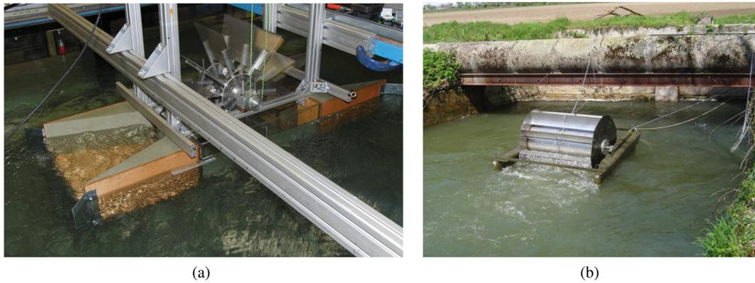
**Fig. 7.** (a) The floating water wheel with the hydrodynamically shaped floating structure, that can convey water to the wheel with minimum head loss (experimental installation, W.M.J. Batten [Batten et al. \(2011\)](#)); (b) example of floating wheel in deep water, real installation (photo of Salmini Santino Elettromeccanica, Italy)
