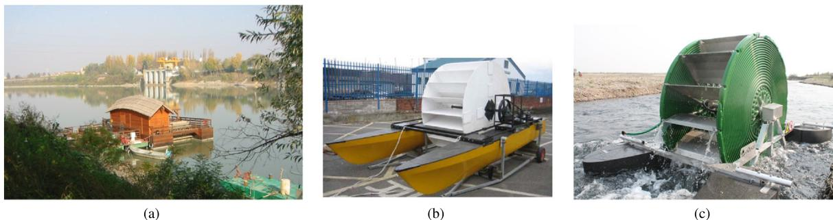
**Fig. 2.** Stream water wheels for different purposes: (a) mechanical power generation (photo courtesy of AIAMS Italy), (b) electricity production Turnock et al., (2007), and (c) pumping in irrigation systems (photo courtesy of Jaime Michavila (Aqysta, n.d.)).
