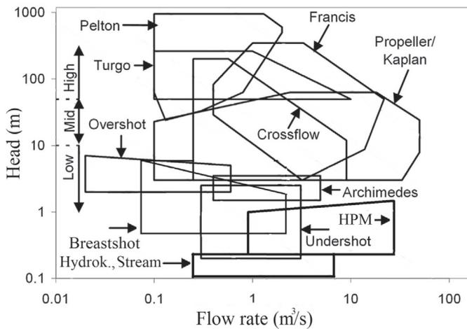
**Fig. 4.** Working conditions of hydropower converters (adapted from Williamson et al., 2014). Stream water wheels and HPM are highlighted with a thicker line, since they were discussed in this review.
