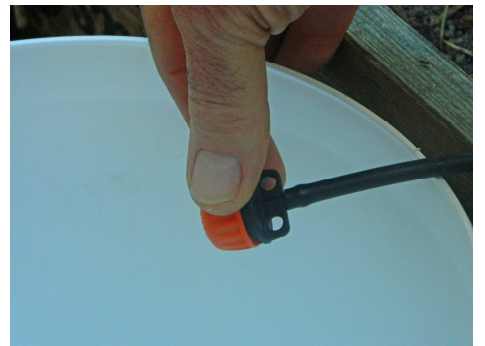
Adjust the control dripper so that flow rate is about the same as the flow rate of the irrigation drippers
