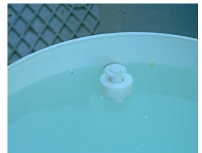
Water level just below the float switch
