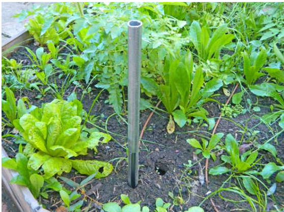
Early in the morning after irrigation the night before, hammer the steel pipe into the soil near a dripper so that the slot face the dripper.
