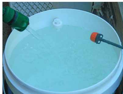
Fill the evaporator with water until the water level is just below the float switch
