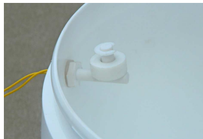
Float switch installed on evaporator with float shaft pointing up
