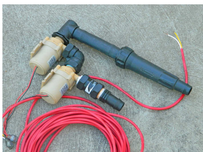
a double pump (two pumps connected in series) with an inlet filter, fittings to connect to 19 mm poly pipe, and 9 metres of waterproof electrical cable
