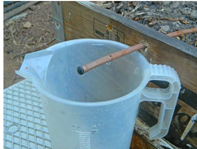
2. Position the measuring container under one of the irrigation drippers so that water drips into the container during the irrigation.
