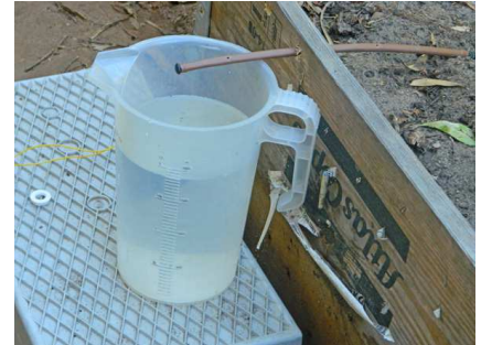
The irrigation stops automatically when the water level reaches the high level
