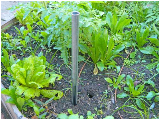
After the irrigation event hammer the steel pipe into the soil near a dripper so that the slot faces the dripper.
