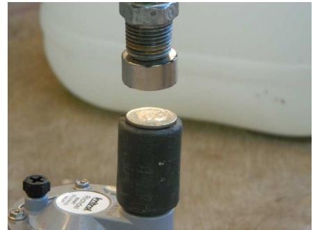
Spacer on top of the solenoid
