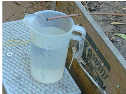
Dripper control volume in the measuring container
