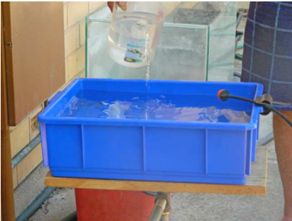
Fill the evaporator with water until the magnet assembly rises
