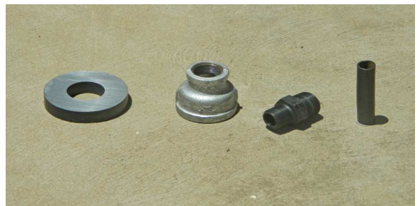
Components of the ferrite ring magnet assembly
