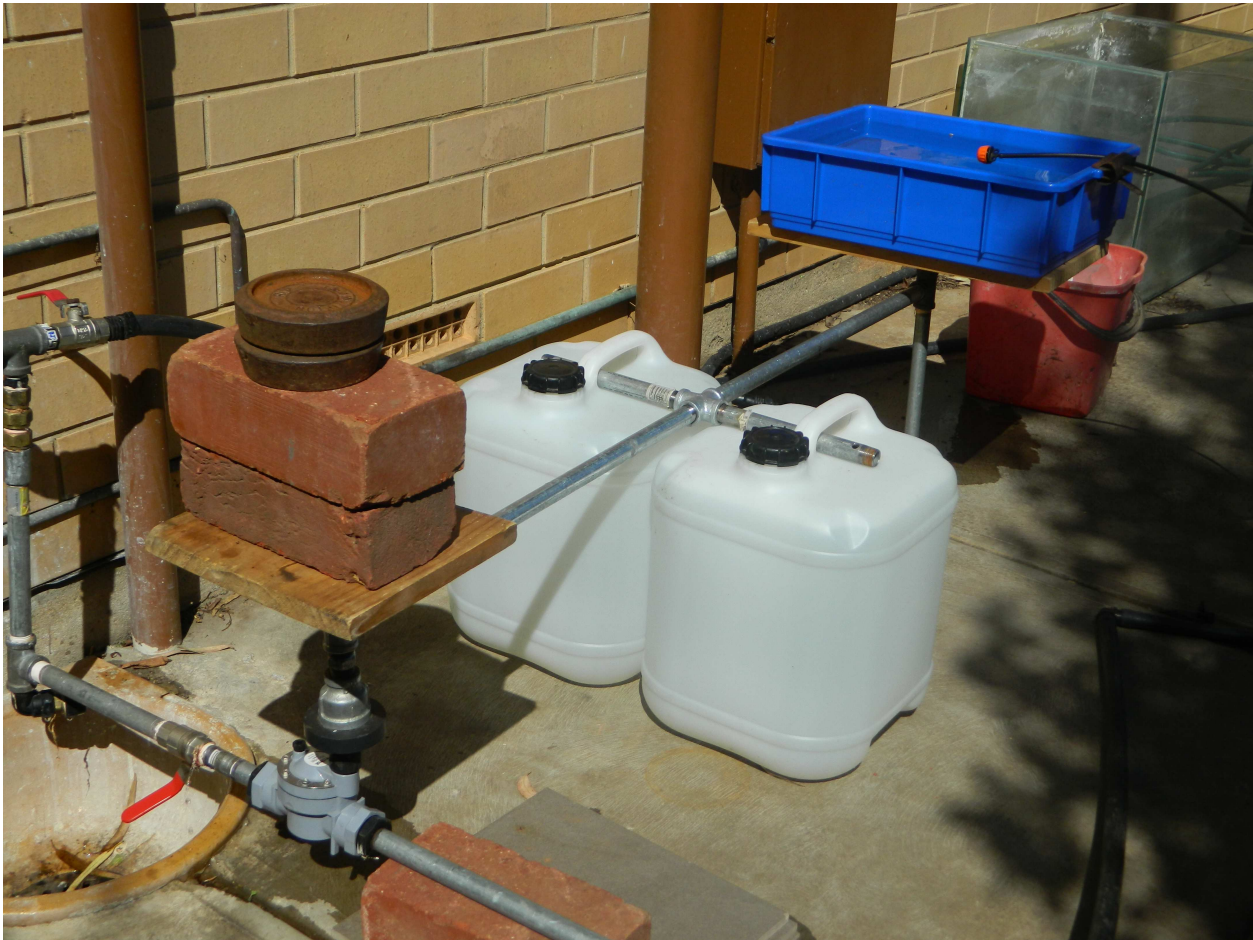
DIY Smart Irrigation Controller with ferrite ring magnet assembly
