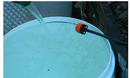
Fill the evaporator with water until the water level reaches the high level
