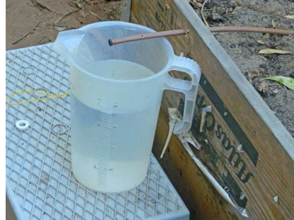
Dripper control volume in the measuring container
