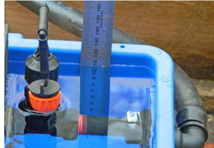
Measure the depth of water in the evaporator at the high level
