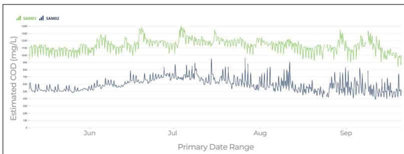
Figure 1: SENTRY™ dashboard with real-time estimated COD (mg/l) values from the influent (SAM01) and primary clarifier effluent (SAM02) sensors.
