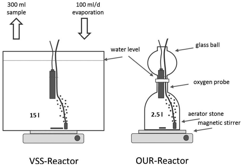
**Figure 3—Experimental setup.**
