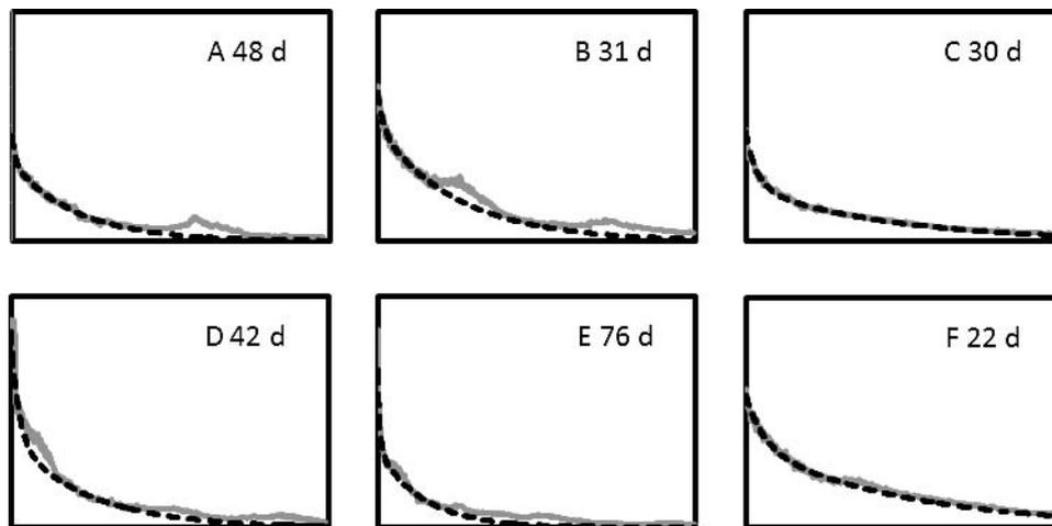
**Figure 4—Respirograms of aerobic digestion batch tests with OUR measured (solid line) and OUR modeled (dashed line); T = duration of experiment; maximum of Y-axis is OUR = 30 mg O<sub>2</sub>/(L·h).**
