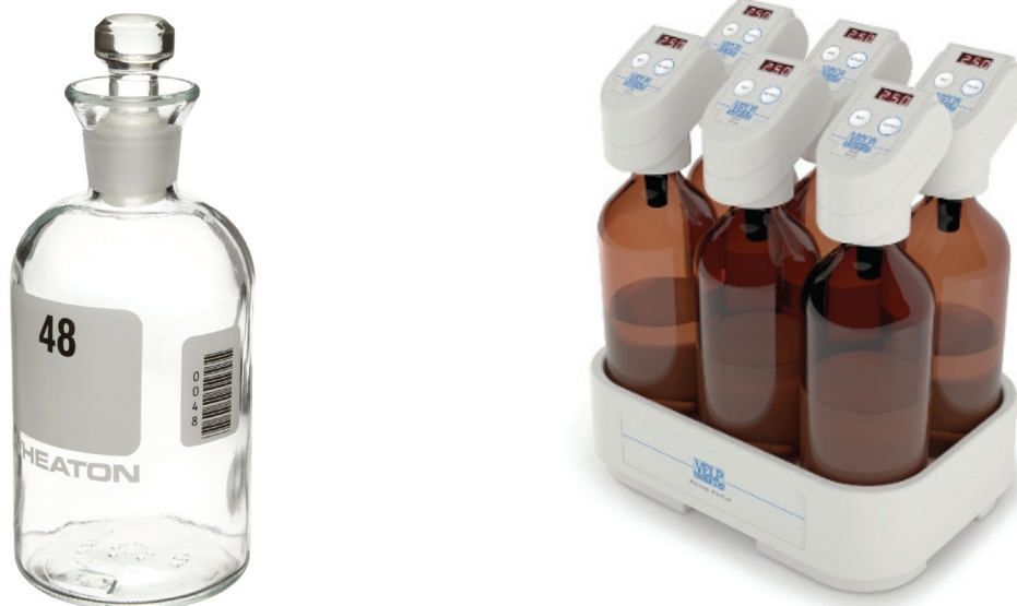
Figure 3.16 A BOD bottle for the classical BOD test (left) and bottles for the continuous measurement of oxygen uptake (right) (photos: Wheaton and Velp Scientifica).
