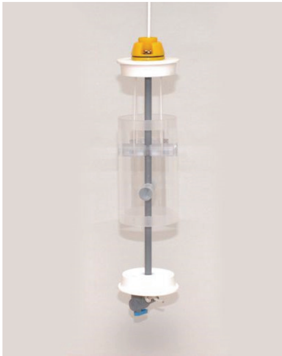
Figure 6.11 A Kemmerer sampler with open upper and lower closures (photo: Royal Eijkelpamp).
