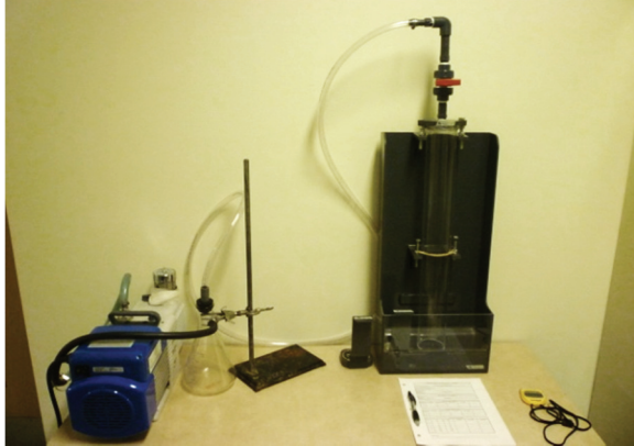
Figure 6.23 ViCAs apparatus with filling equipment (photo: Gromaire M.C. and Chebbo G., ViCAs manual).
