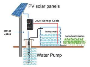
Operation principle is to convert the energy from Solar Radiation to Mechanical Energy of motor-shaft to pump water at specified flow-rate in the head.
