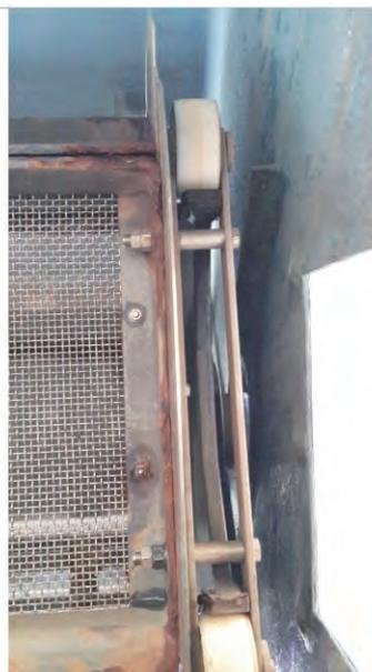
Stainless mesh plates to lift up small screenings, 3mm of opening
