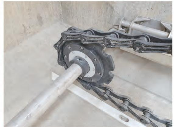
Head sprockets, Driven sprockets, Take up sprockets
