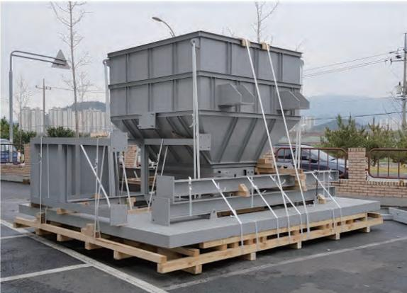
Slide gates opens by power cylinders. 4 road cells installed.
