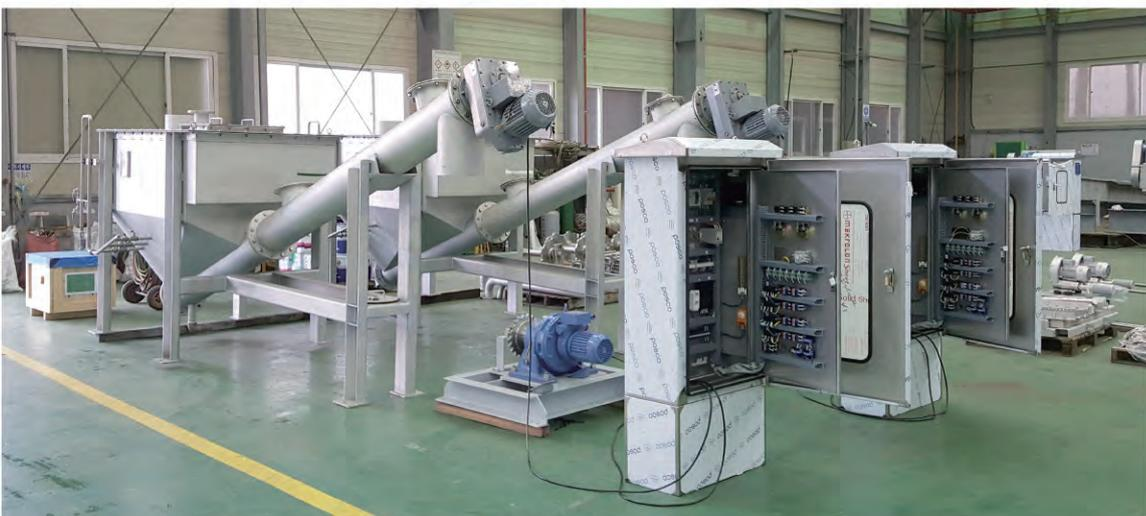
PLC testing for 2 automatic grit separators for Viet Tri Wastewater Treatment plant in Vietnam.
