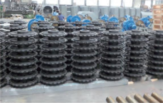
Cast iron sprockets and steel flights tar epoxy coated
