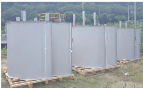
Center feed well made of stainless steel
