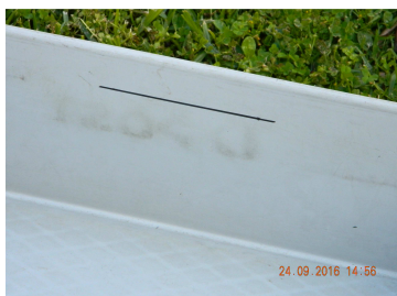
Level line on inside of evaporator
