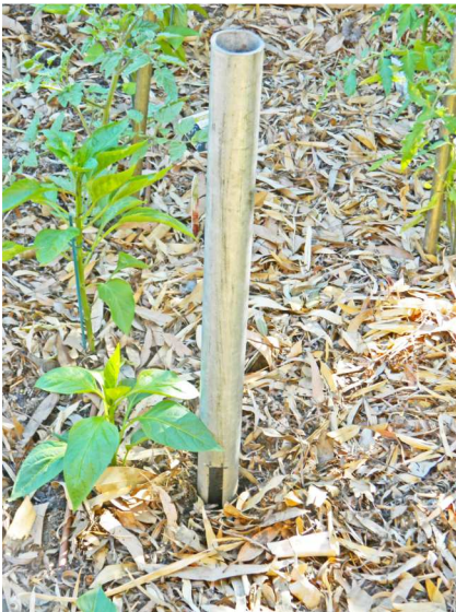
Early in the morning after irrigation the night before, hammer the steel pipe into the soil near a dripper
