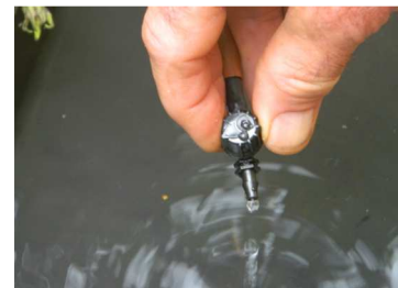
Increase the flow rate of the adjustable control dripper to reduce water usage
