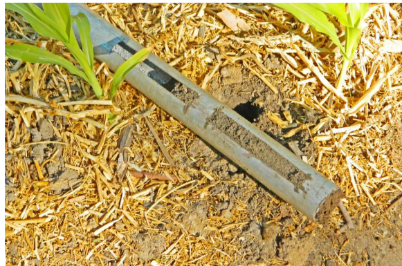
Remove the steel pipe from the soil and use the slots to inspect the moisture level in the soil and the position of the wetting front
