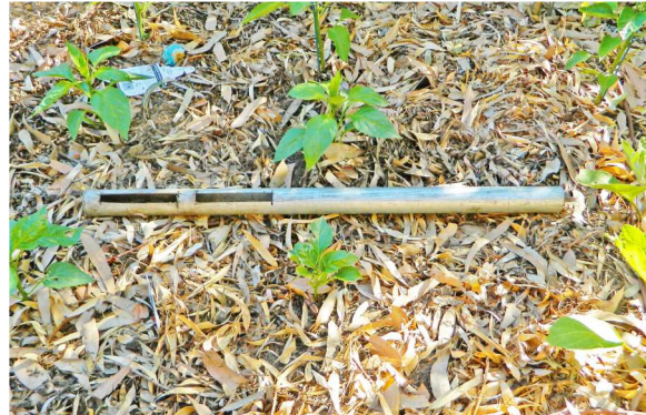
An angle grinder can be used to make some slots in a length of steel pipe
