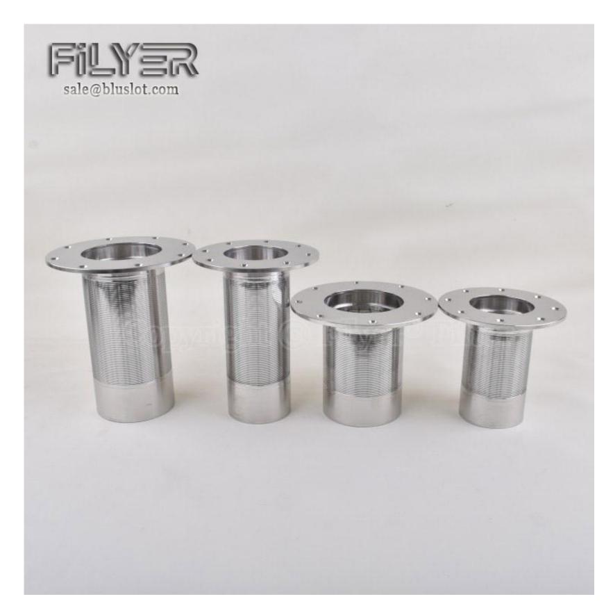
On the water system pipeline near the outlet of equipment containing resin such as ion exchangers, install a resin trap filter screen with a hole diameter much smaller than that of the resin. It also has a flushing function. When the resin passes through, it can be intercepted and captured by the filter screen.
