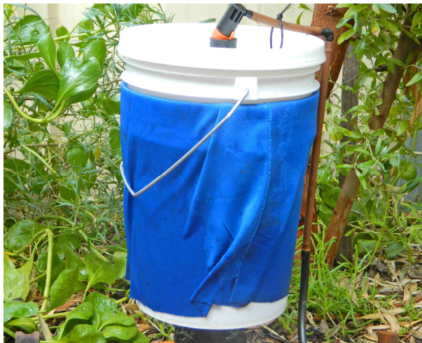
A polyester cloth wicks water from inside the bucket to outside the bucket to evaporate
