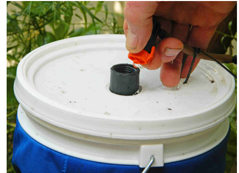
Adjusting the control dripper
