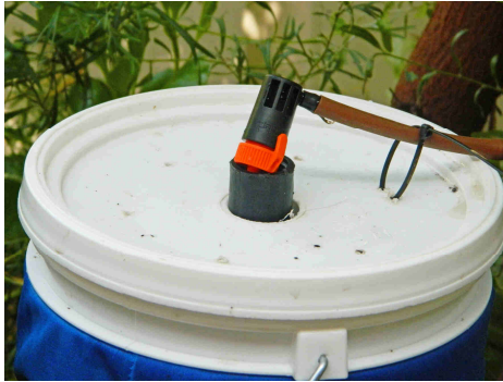
Rainwater enters the bucket via the six small drain holes in the lid
