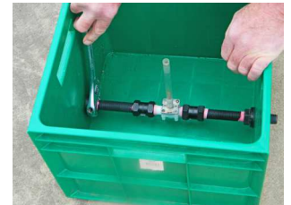
Tighten the internal backing nuts against the external round plastic nuts
