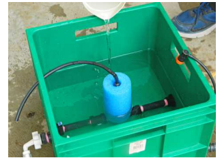
Fill the evaporator with water until the float jumps up
