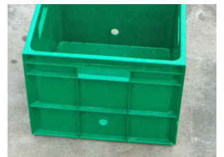
Drill 2 holes in opposite sides of the evaporator
