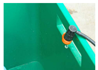
Adjust the control dripper so that water drips into the evaporator
