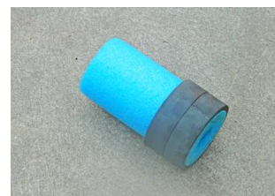
8 cm diameter float with two float rings
