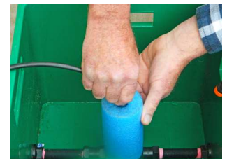
Connect the overflow tube to the top of the float shaft
