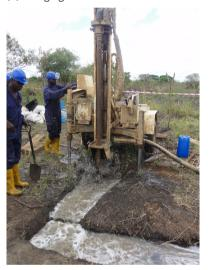
Viscous drill mud is pumped down the drill pipe, emerging at the bit and washing cuttings up the hole. As with the manual techniques of jetting and sludging, mechanized (direct circulation) mud rotary drilling relies on the hydrostatic pressure of the fluid in the borehole to prevent collapse.
