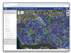
All water supply, drainage, and coastal systems are modeled in an integrated way and visualized in a web GIS environment.
