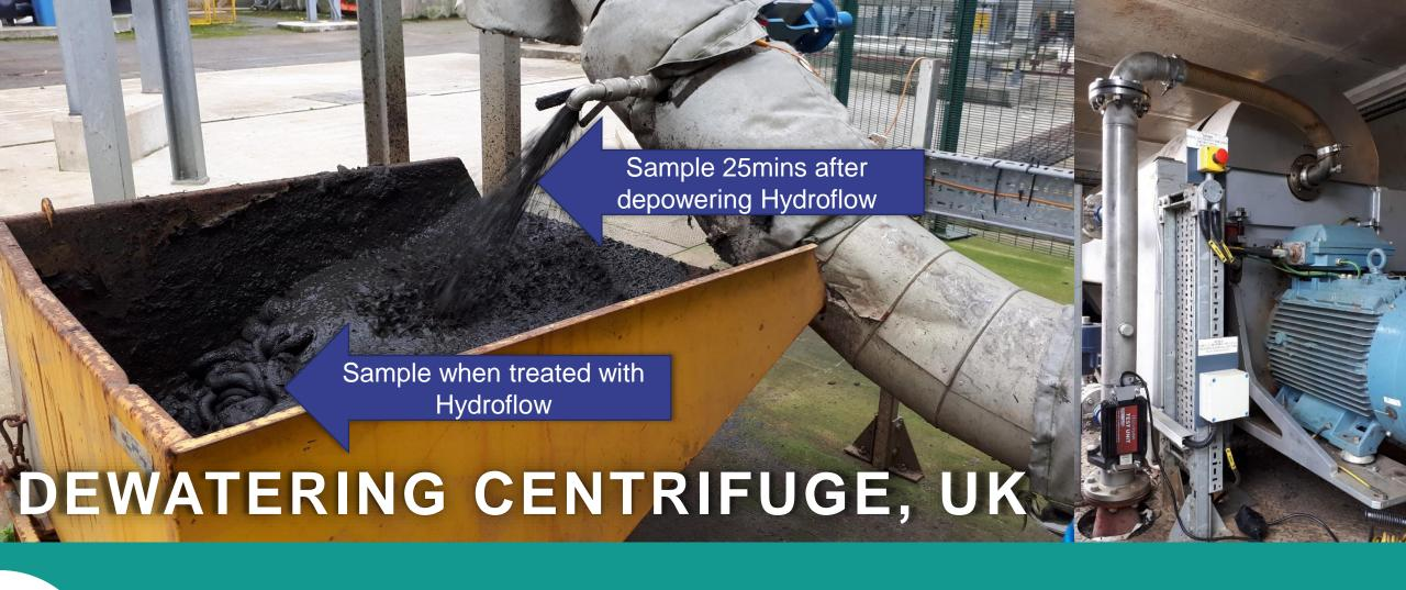
Comparing parallel centrifuges, (same torque) polymer reduction from 3.5 to 3.1 kg/ tDS Comparing same centrifuge, (const. torque) polymer reduction from 3.6 to 3.2 kg/ tDS Turning off Hydroflow results in visible change to samples in <25min HydroFlow
