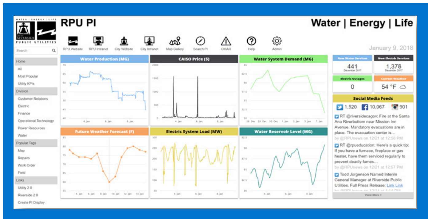
Figure 3: Riverside Public Utility provides a single web interface that any user can drill down into to see what is happening in real time.
